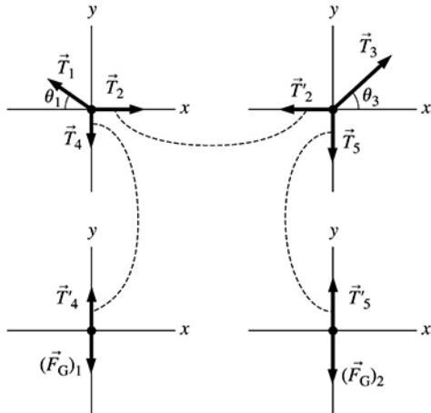
**Solve:** (a) We will consider both the two hanging blocks *and* the two knots. The blocks are in static equilibrium with  $\vec{F}_{\text{net}} = 0 \text{ N}$ . Note that there are three action/reaction pairs. For Block 1 and Block 2,  $\vec{F}_{\text{net}} = 0 \text{ N}$  and we have
